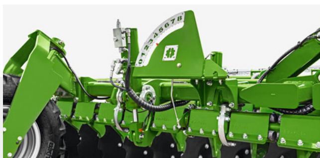
Hydraulic working depth adjustment with easy-to-read scale
